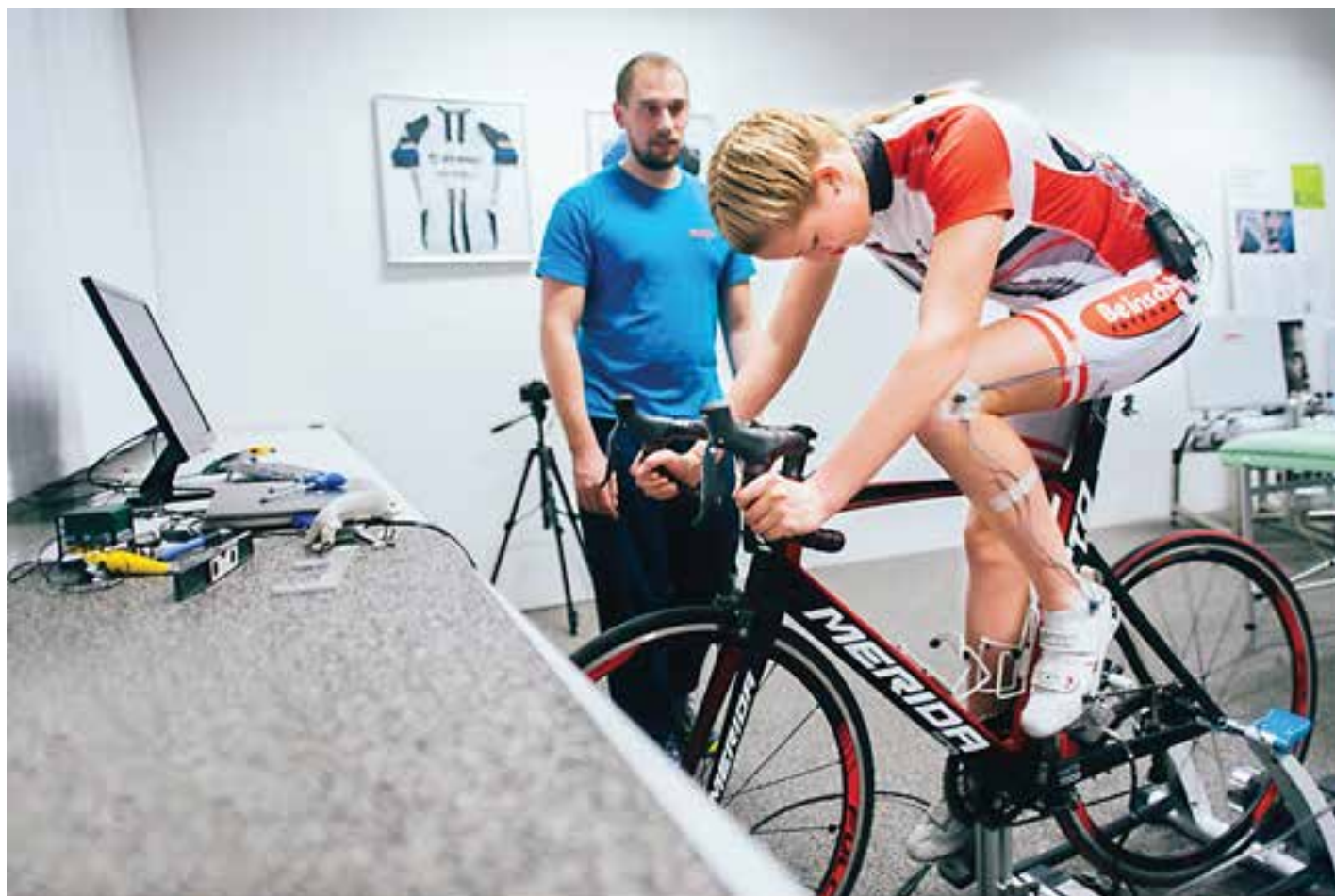
Figure 7: Modern bike fitting is an interactive process incorporating data from a variety of sources such as three-dimensional motion analysis, shoe and saddle pressure distribution and pedal force application.
